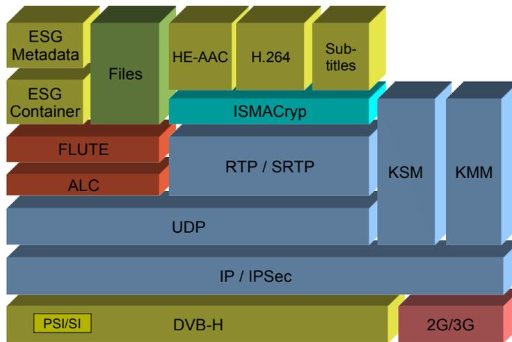
Figure 3: IP Datacast over DVB-H Protocol Stack Architecture (indicative) [1]
