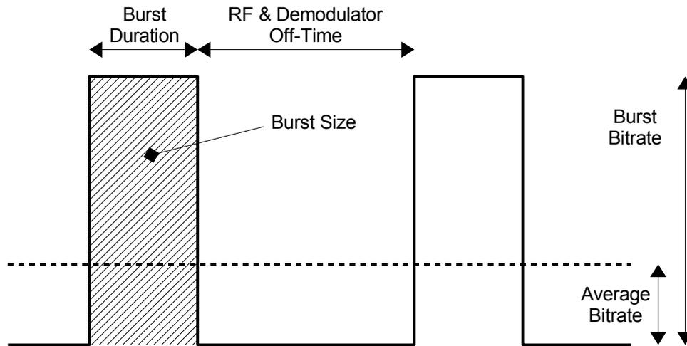
Figure 1: Principle of Time-Slicing [2]
